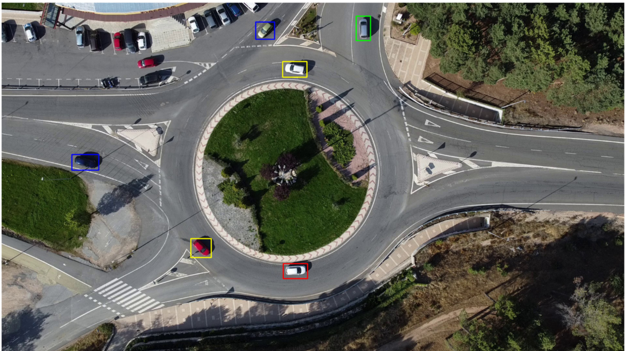
Figure 15. Vehicles belonging to each area (blue: entrance, green: exit, yellow: circulating traffic, red: rest).
