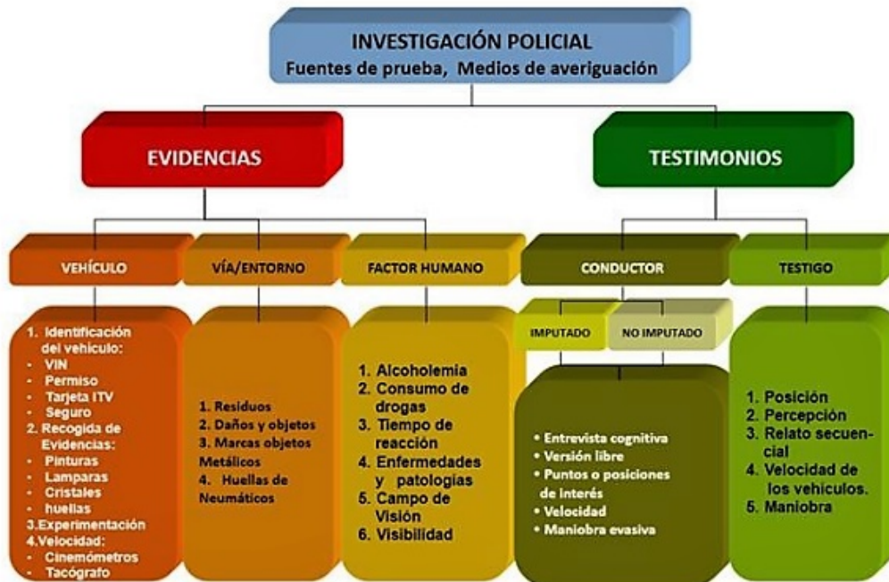
Figure 5. Diagram of the sources of evidence to be collected in a road accident. Source: (Campón, 2019)
