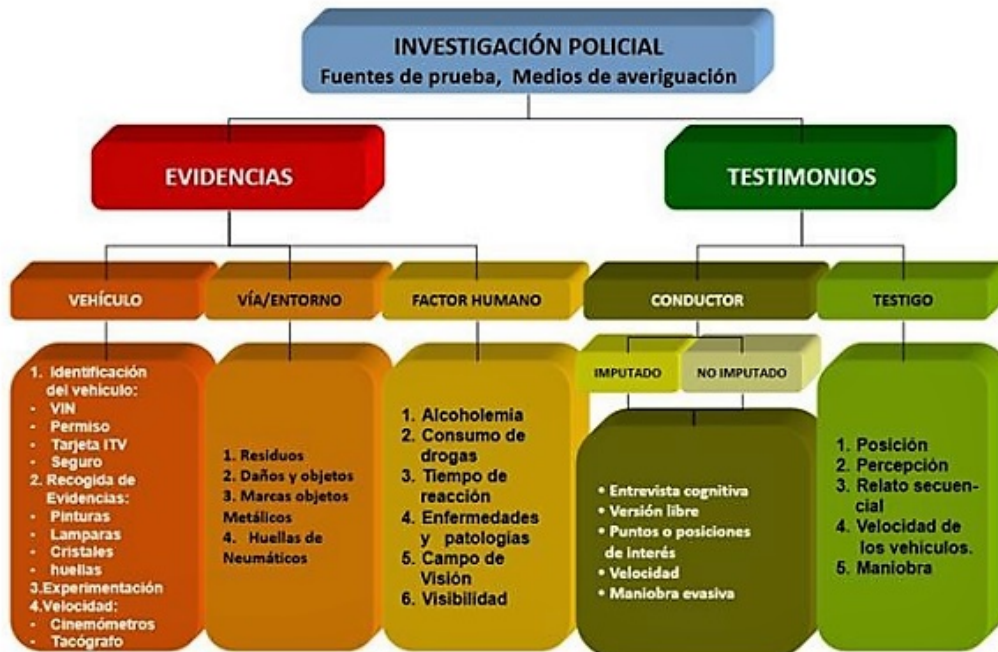
Figure 5. Diagram of the sources of evidence to be collected in a road accident. Source: (Campón, 2019)
