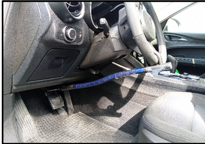
Image no. 7: Fitting the “steering wheel-pedal clamp” type immobiliser to a vehicle. Source: Prepared internally.
