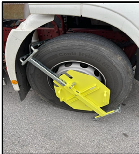
Image no. 8: Fitting the wheel clamp immobiliser on a lorry. Source: Prepared internally.
